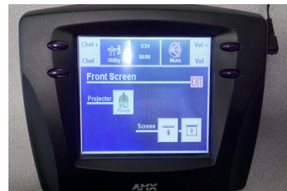
Figure 1 The AMX control panel
